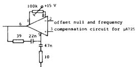
Fig. 2. Circuit diagram of the complete amplifier. For a description see text. All resistances 'R' have the value 47 K $\Omega$ . Amplifier modules: 1. Low cost version where low noise is not of prime importance:  $A_1$  – CA3130 (RCA);  $A_3$ ,  $A_4$  – low offset –  $\mu$ A725 (Fairchild);  $A_2$ ,  $A_5$ – $A_{10}$  – AD74! (Analog Devices). 2. Low noise version:  $A_1$  – 3523 (Burr Brown);  $A_2$ ,  $A_{10}$  – OP-05 (Bourns);  $A_3$ – $A_9$  –  $\mu$ A725 (Fairchild).
